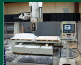
5-Axis CNC Router for Fast, Accurate and Less Costly Pattern Making
