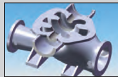
Resulting 3D model from a scan of an old pump at a customer's location.
