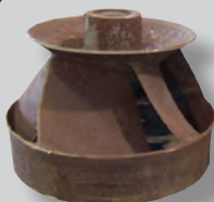
Old worn impeller
