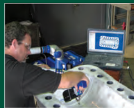
Laser Scanning of Sample Casting
