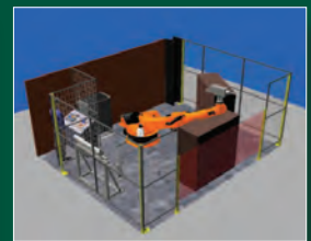
CNC Robotic Sand Milling Cell. Patternless Molding. Faster turnaround time than conventional tooling requirements.
