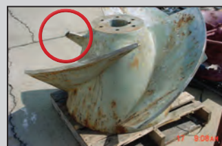
○ Broken Impeller Vanes
